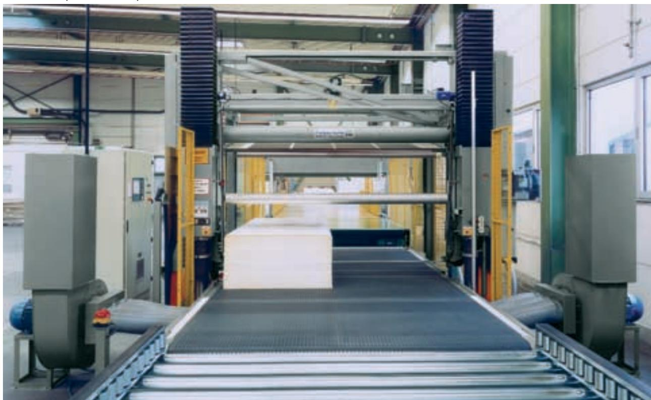
Automatic Horizontal Splitting and Stacking Machine H 52
