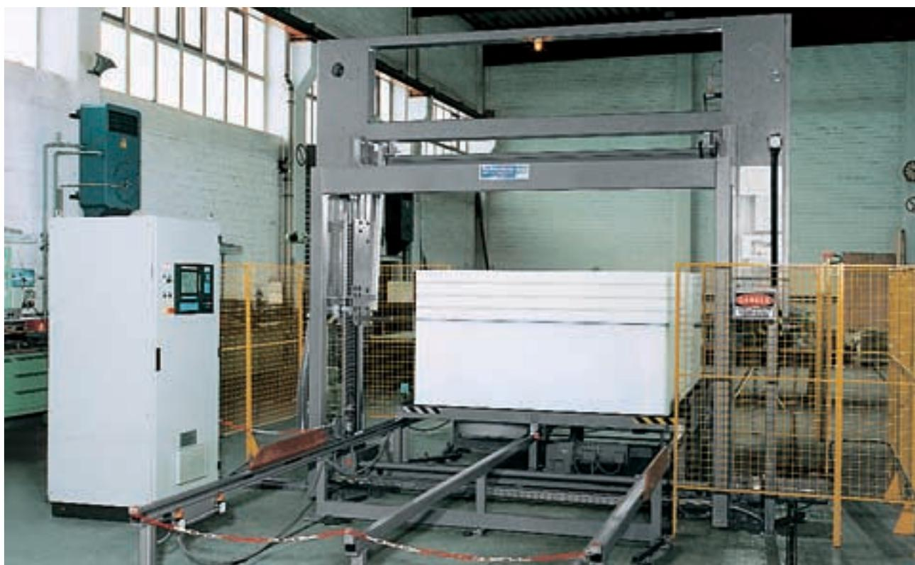
Automatic Horizontal Splitting and Stacking Machine W 21 with sliding table
