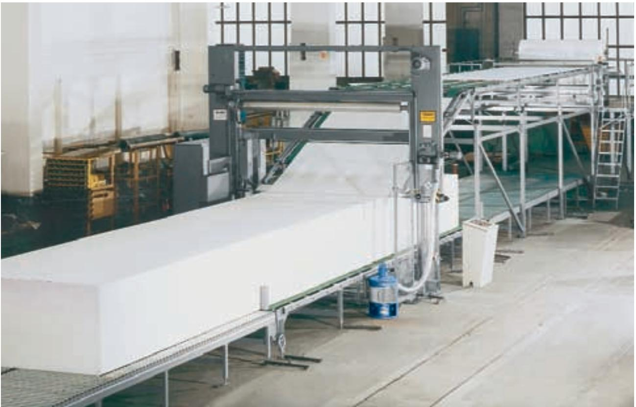
Machine W 22 with conveyor belt and wind-up machine A 2
